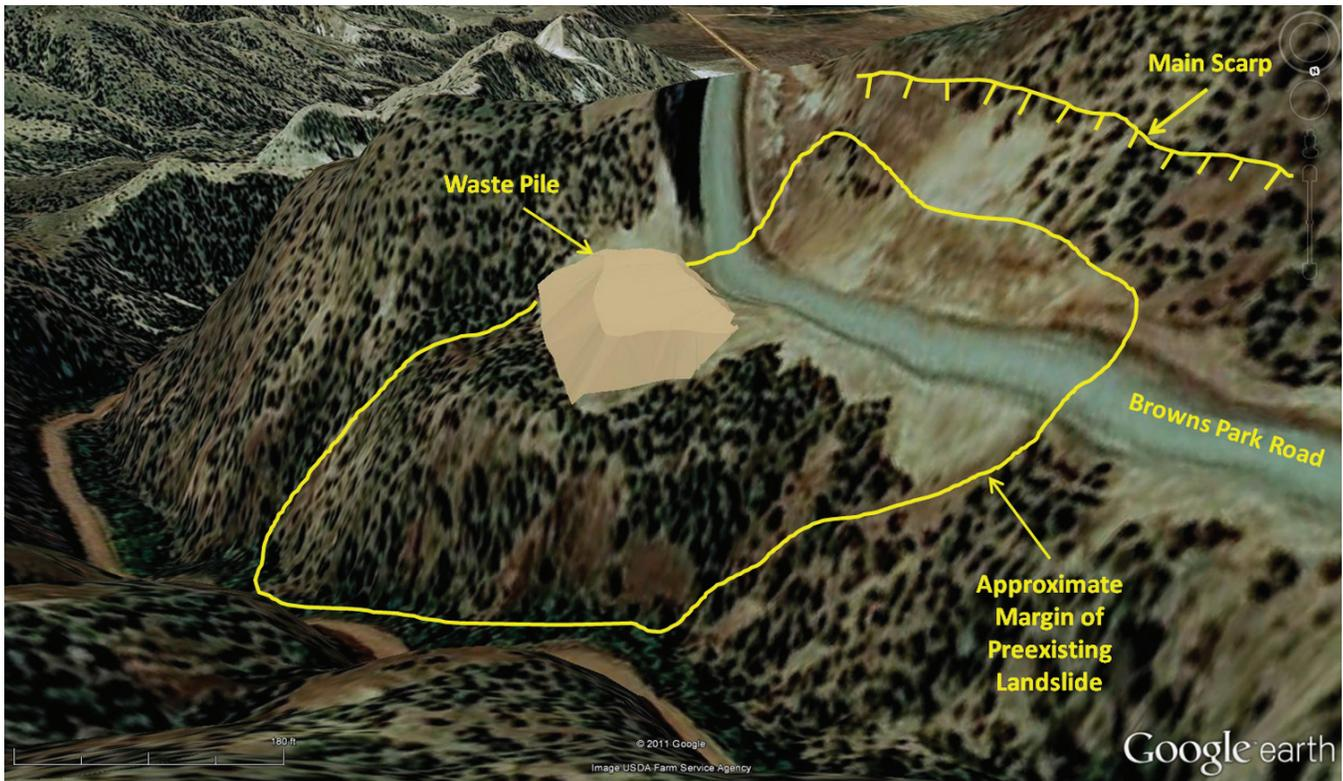
**Figure 7.** Oblique view, looking south, of preexisting landslide and waste pile. Waste pile was constructed on top of a back-tilted surface created during previous landslide movement. Google Earth image from 2009 National Agriculture Imagery Program.
