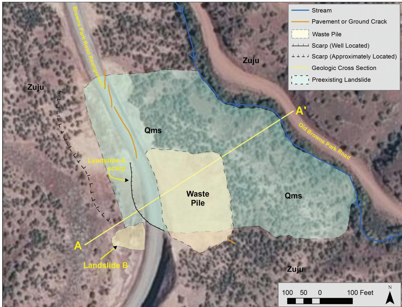
**Figure 5.** Map of preexisting landslide, Landslide A scarp, and waste pile. Geologic cross section A–A' is shown on figure 8. Geologic units include landslide debris (Qms) and Upper Jesse Ewing Canyon Formation shale interbedded with quartzose and lithic sandstone (Zuju). Bedrock geology from Sprinkel (2006) and landslide and waste pile extents from this reconnaissance. Base from 2009 National Agriculture Imagery Program.
