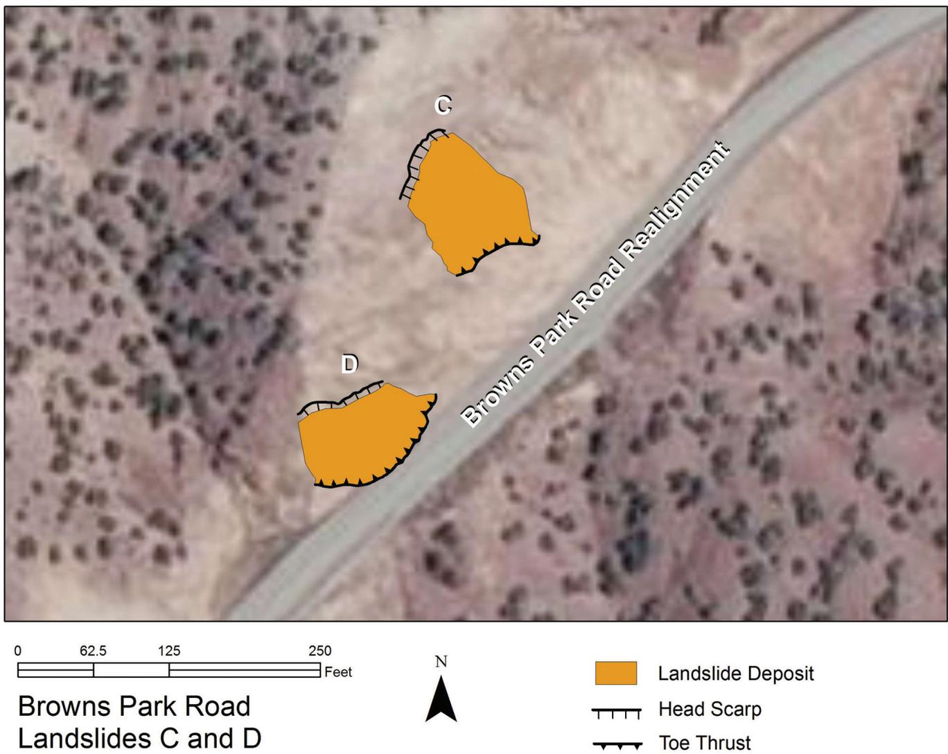
**Figure 9.** Locations of Landslides C and D. Both landslides are translational rockslides on a  $34^\circ$  (1.5H:1V) cut slope above Browns Park Road. Landslide D impacted a guardrail and filled the small roadside drainage ditch. Base from 2009 National Agriculture Imagery Program.
