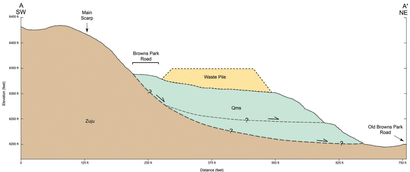
**Figure 8.** Geologic cross section of preexisting landslide. Surface profile based on DEM of the pre-road realignment landscape. Bounds of preexisting landslide (Qms) and waste pile are from geologic mapping conducted during this reconnaissance. Landslide (Qms) overlies intensely fractured and weathered shale, sandstone, and siltstone with minor lenses of silicic conglomerate (Zuju). See figure 5 for cross section line location.
