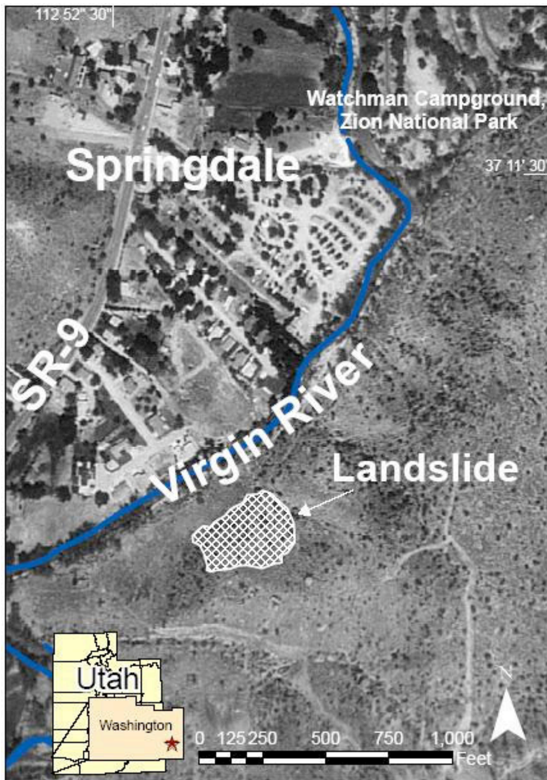
Figure 2. Rotational slump landslide formed during May 2005 on the east side of the Virgin River in Springdale, Utah (base map U.S. Geological Survey Springdale East 7.5' orthophoto quadrangle).
