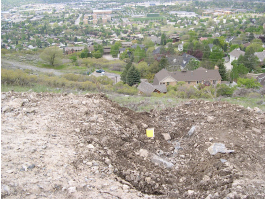
Figure 7. Impact crater (bounce mark) on the slope just above the guest house (yellow object is notebook for scale).
