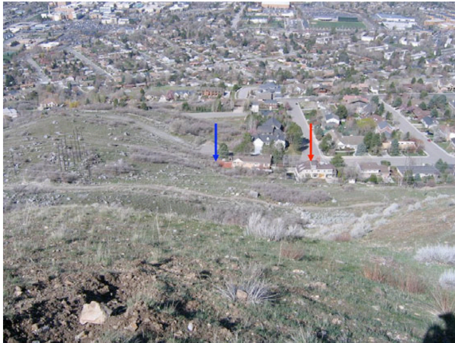
Figure 9. Previous guest house location destroyed by the 2005 rock fall (blue arrow) and the house damaged by the 2009 rock fall (red arrow). Rock-fall boulders on the alluvial fan left of the blue arrow and the slope above the impacted houses show the distribution and size of historical and prehistorical rock fall and the proximity of houses to the hazard.
