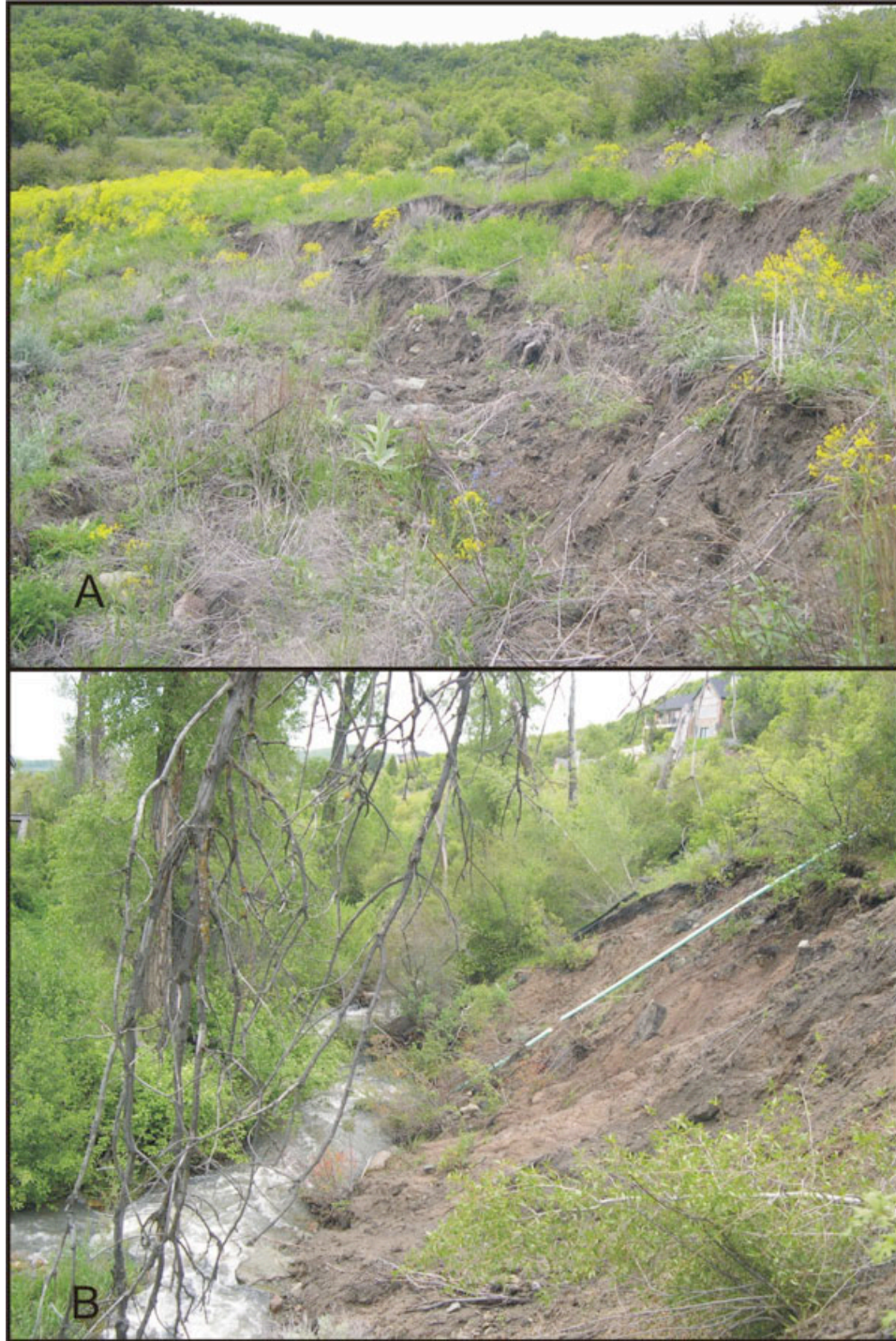
Figure 4. Northern Sewer-Line landslide. (A) View to the south-southwest of main scarp zone of the landslide. Top of main scarp was only a few feet from the east edge of the sewer-line corridor. (B) View to the south of toe of the landslide along Gordon Creek. Note drainpipe exposed along south flank of landslide.
