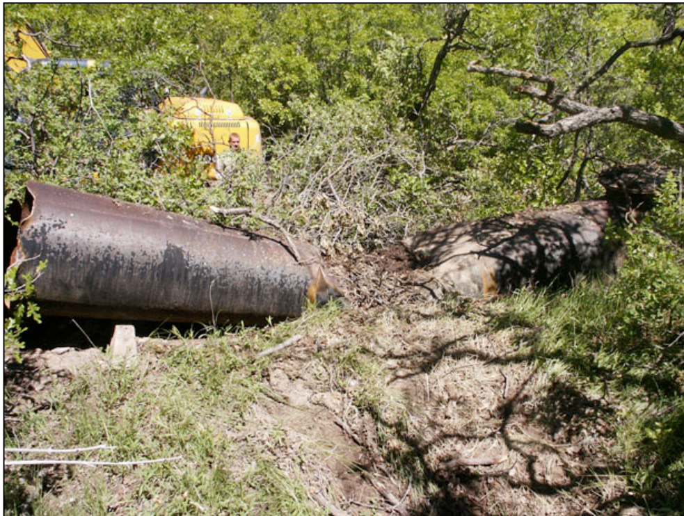
Figure 7. Ruptured Parowan City penstock where it was struck by a second rock-fall boulder weighing approximately 10 tons. After striking the penstock, the boulder continued toward Parowan Creek for an additional approximately 50 feet.
