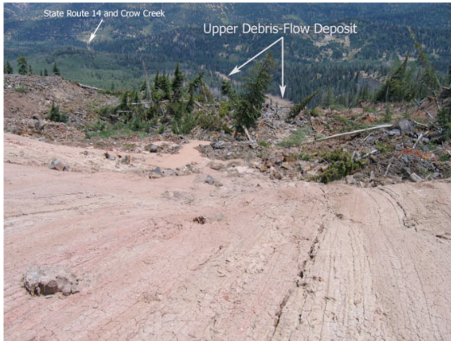
Figure 7. View from the landslide main scarp toward Crow Creek and SR-14. The main scarp is covered with slickensides. The debris-flow path and deposits are evident in the unnamed tributary stream valley to Crow Creek.
