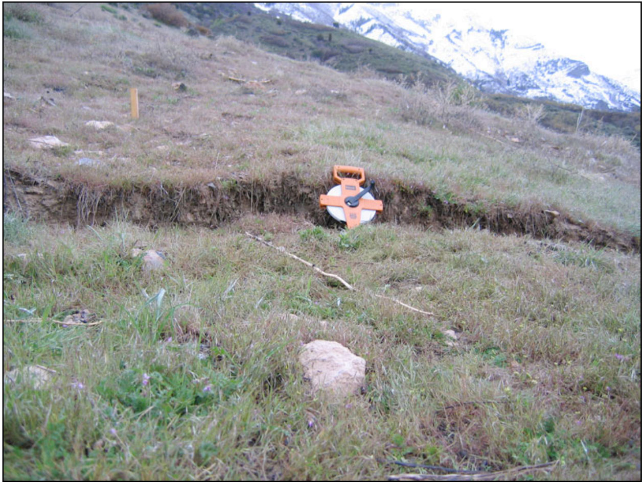
Figure 13. View of main scarp of small landslide upslope of main slide on May 12, 2005. By May 5, 2005 another scarp connected this small slide to one farther upslope joining the two slides into a single shallow landslide.
