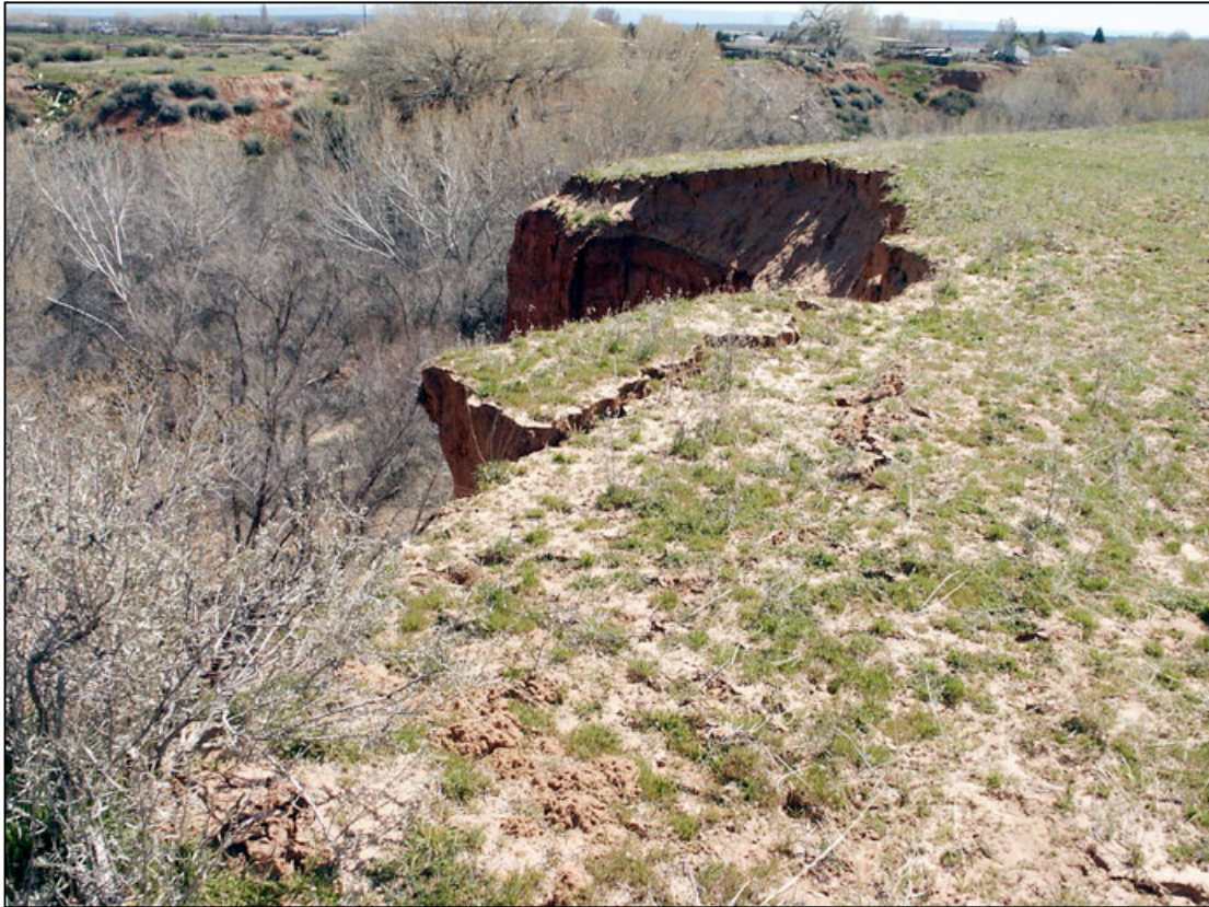
Figure 6. Partially detached section of the arroyo wall where additional failure is imminent.
