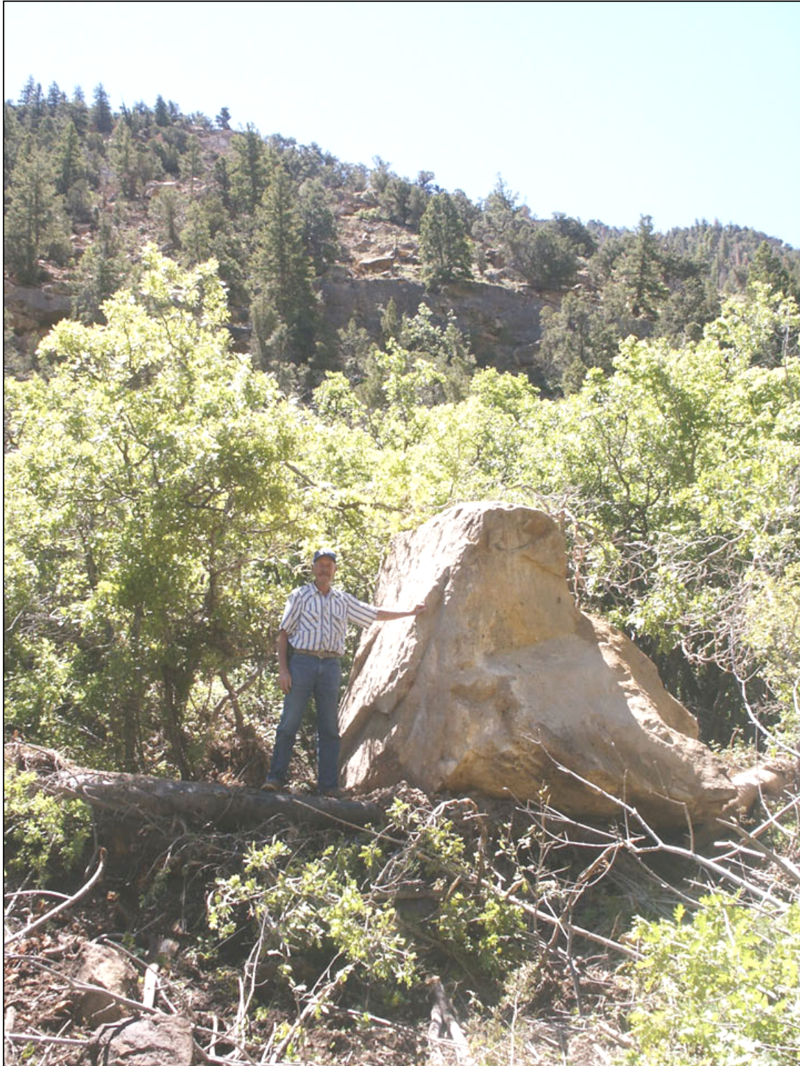
Figure 5. Sandstone boulder weighing an estimated 80 tons resting directly on top of a section of the Parowan City penstock. The rock-fall path down the east wall of Parowan Canyon is visible through the trees below the skyline.
