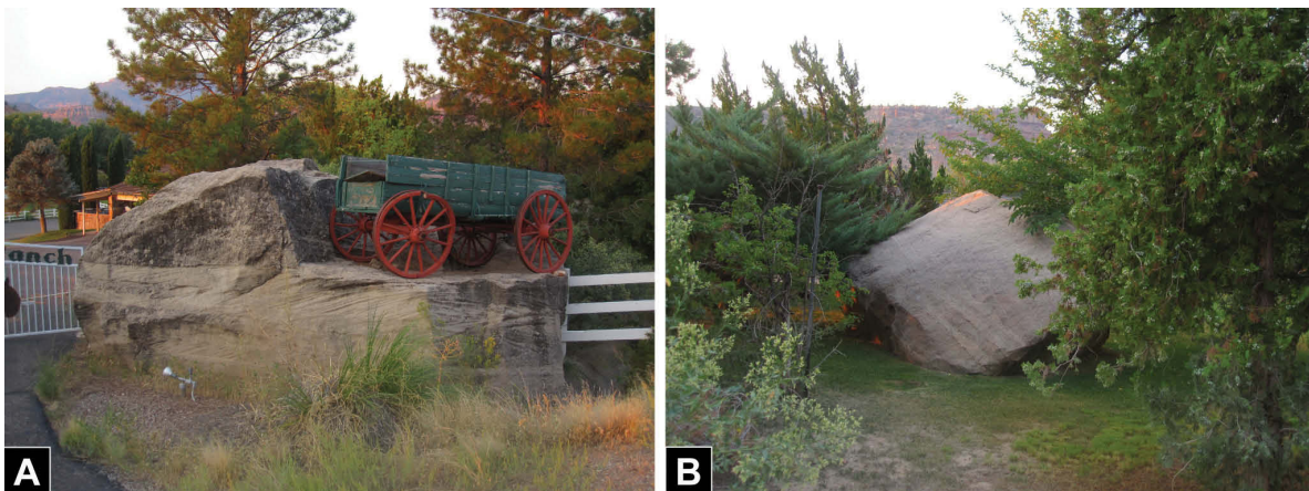
Figure 13. Rock-fall boulders at the Rock-N-River Ranch. Both photos taken September 29, 2010; views are to the south. A. Approximately 20 x 17 x 10-foot boulder that reportedly rolled across SR-9 in 1976. B. Approximately 18 x 10 x 10-foot boulder lying about 50 feet to the west that may have fallen at the same time.
