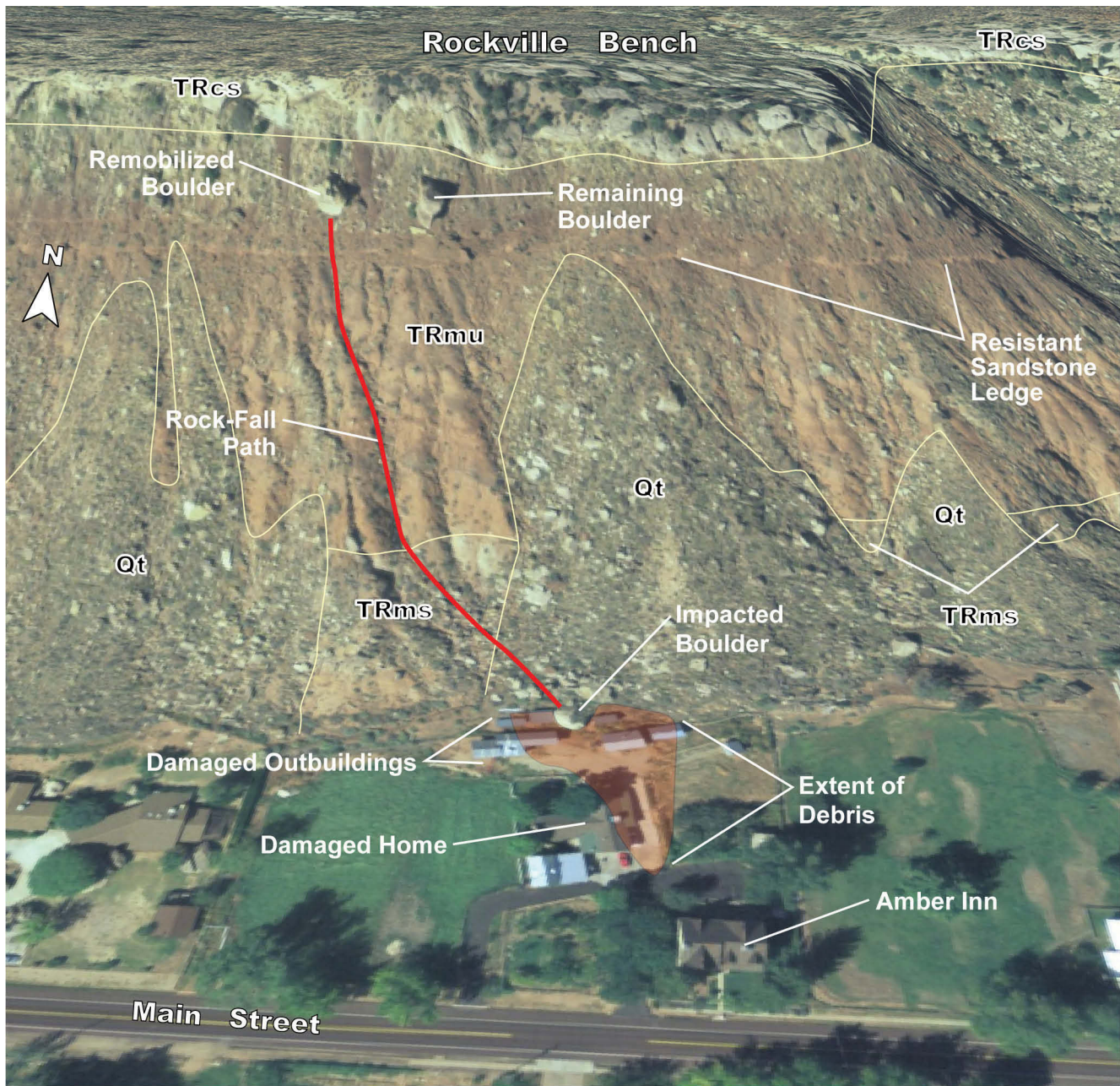
Figure 3. Three-dimensional model of the February 2010 rock-fall site constructed by draping 2006 HRO imagery over a 10-meter-resolution digital elevation model. Rock-fall source area, path (red line), extent of post-impact debris, and damaged structures are shown. Rockville Bench geology modified from Willis and others (2002): TRcs = Shinarump Conglomerate Member of the Triassic Chinle Formation, TRmu = upper red member of the Triassic Moenkopi Formation, TRms = Shnabkaib Member of the Moenkopi Formation; Qt = Quaternary talus deposits.
