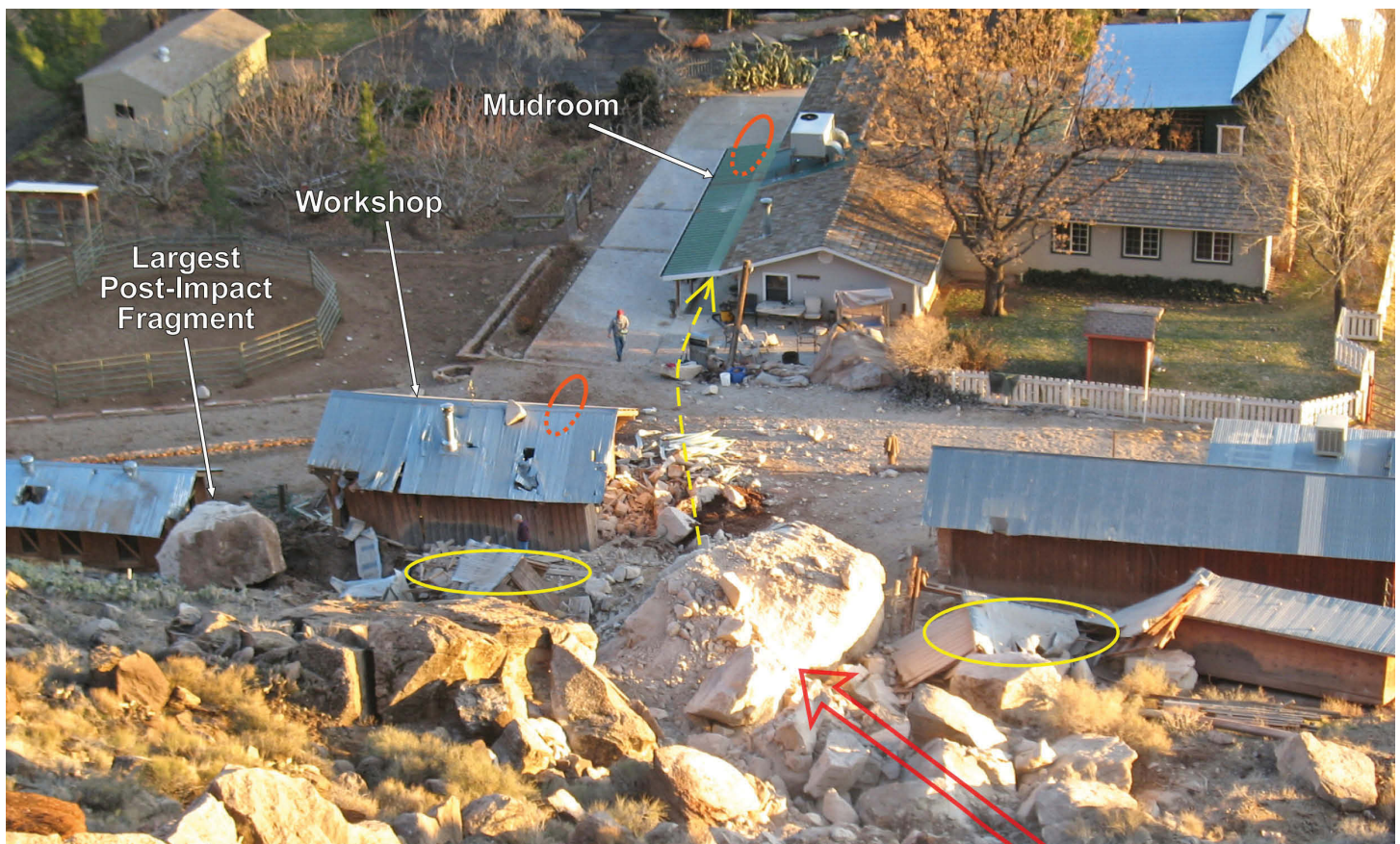
Figure 4. View to south of impact area and property damage at 274 West Main Street; photo taken on February 10, 2010. Red arrow indicates the path traveled by the rock-fall boulder to the area of impact with a previously fallen boulder. Yellow ellipses show locations of destroyed sheds. Red ellipses show the approximate locations of damaged vehicles before they were removed. Yellow dashed arrow shows travel path of a large fragment that damaged the house and a parked vehicle.
