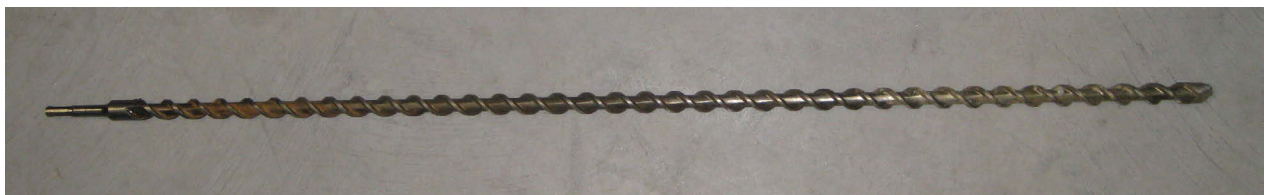
Figure B2. SDS plus, 37-inch-long (39 inches with shank), 3/4-inch-diameter masonry bit.
