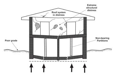
Figure 6.1. Typical structural damage to a building from expansive soil (modified from Black and others, 1999).
