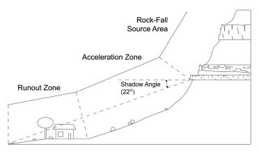
Figure 3.5. Components of a characteristic rock-fall path profile (from Castleton, 2009).
