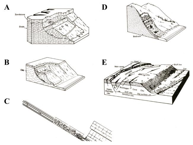
Figure 4.3. Examples of rotational and translational landslides: (a) rotational rock slide, (b) rotational earth slide, (c) translational rock slide, (d) debris slide, and (e) translational earth slide mass (from Cruden and Varnes [1996], Special Report 247: Landslides—Investigation and Mitigation, figure 3-22, p. 57. Copyright, National Academy of Sciences, Washington, D.C.; reproduced with permission of the Transportation Research Board).
