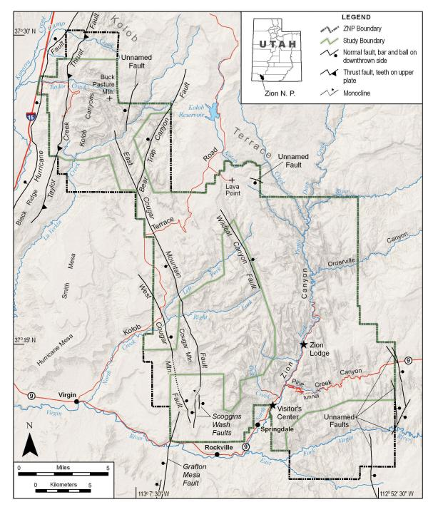
Figure 5.5. Normal and thrust faults in the Zion National Park Geologic-Hazard Study area.
