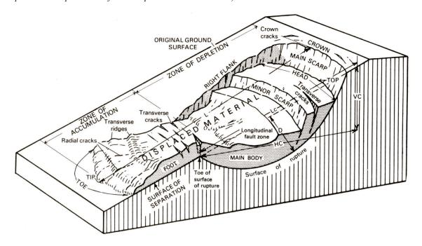
Figure 4.4. Block diagram of an idealized complex earth slide (from Cruden and Varnes [1996], Special Report 247: Landslides—Investigation and Mitigation, figure 3-2, p. 40. Copyright, National Academy of Sciences, Washington, D.C.; reproduced with permission of the Transportation Research Board).
