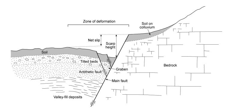
Figure 5.3. Cross section of a typical normal fault showing scarp formation, tilted beds, and graben formation in the deformation zone associated with the fault (modified from Robison, 1993).
