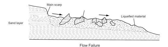
Figure 5.7. Four principal types of liquefaction-induced ground failure; arrows indicate direction of movement (modified from Youd, 1984; Harty and Lowe, 2003).
