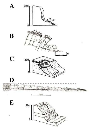
Figure 4.2. Types of landslides: (a) fall, (b) topple, (c) slide, (d) spread, and (e) flow. Broken lines indicate original ground surfaces; arrows show portions of trajectories of individual particles of displaced mass (from Cruden and Varnes [1996], Special Report 247: Landslides—Investigation and Mitigation, figure 3-19, p. 53. Copyright, National Academy of Sciences, Washington, D.C.; reproduced with permission of the Transportation Research Board).
