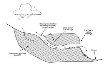
Figure 6.7. Cross section of a pipe in fine-grained Holocene alluvium (after Black and others, 1999).
