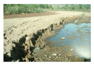
Figure 5.8. Lateral-spread cracking from liquefaction along the Virgin River resulting from the September 2, 1992, M 5.8 St. George earthquake. Folding shovel for scale (photo credit W.E. Mulvey).
