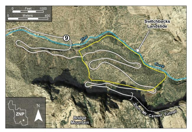
Figure 4.6. Zion-Mount Carmel Highway Switchbacks landslide (image source 2006 National Agricultural Imagery Program).
