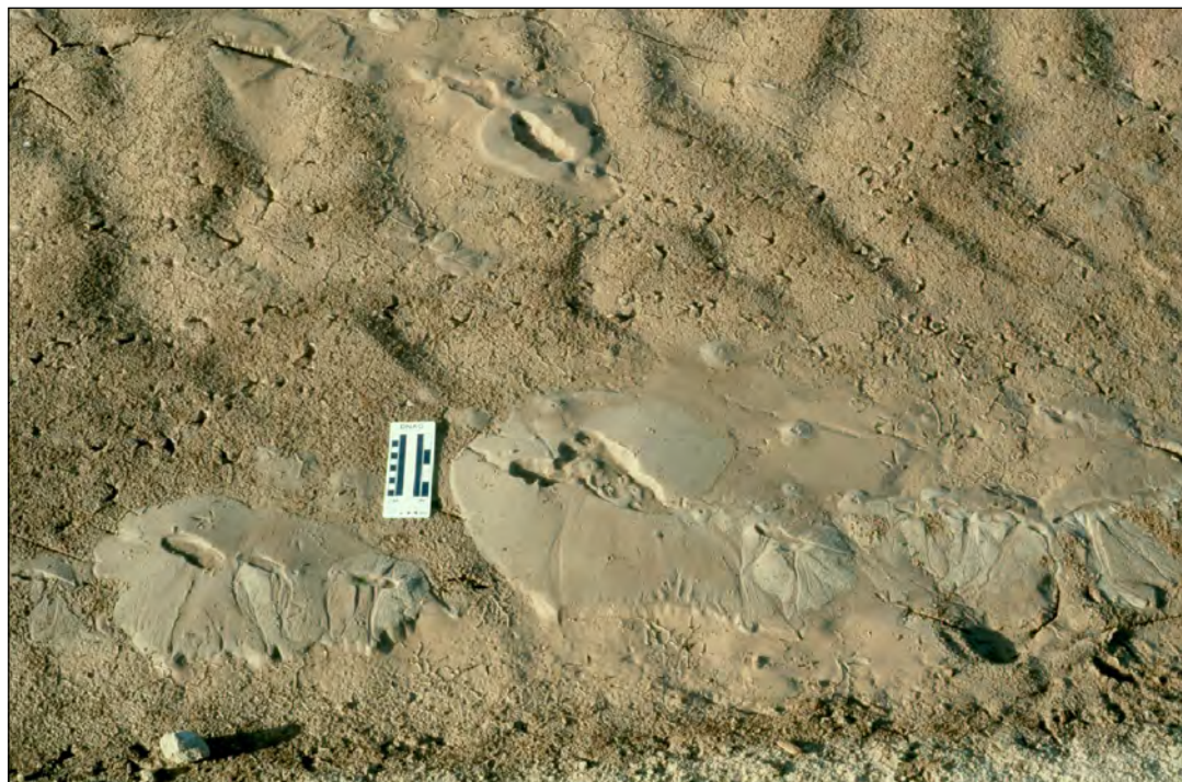
Figure 3. Sand blows from liquefaction along the Virgin River resulting from the September 2, 1992, M 5.8 St. George earthquake. Scale card shows centimeters (left) and inches (right) (photo credit W.E. Mulvey).
