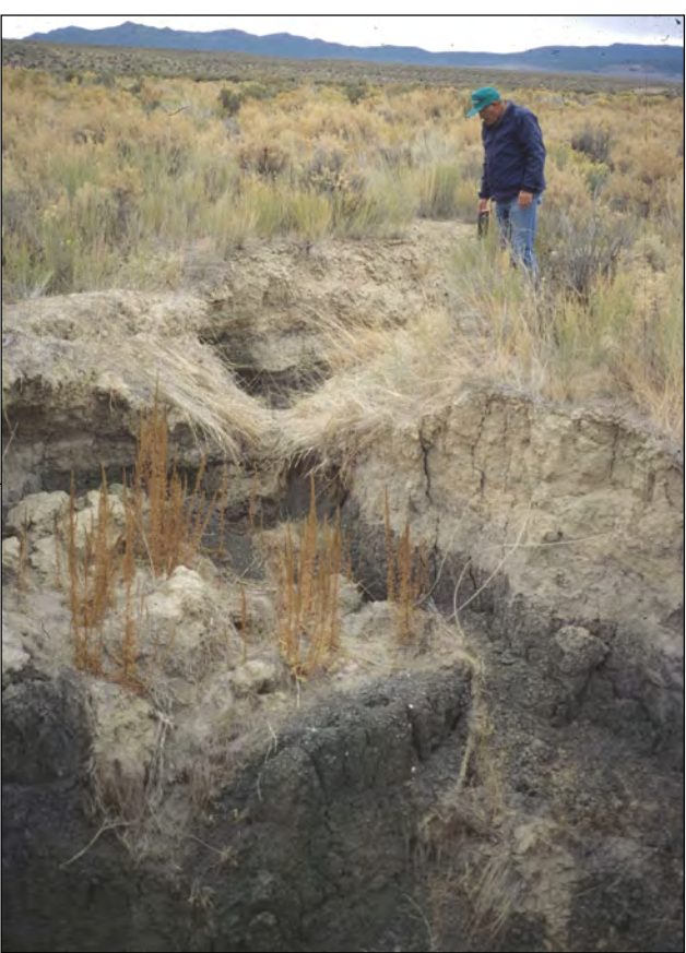
Figure 2. Collapsed pipe in fine-grained floodplain alluvium in southwestern Utah. Photo date: October 2005.
