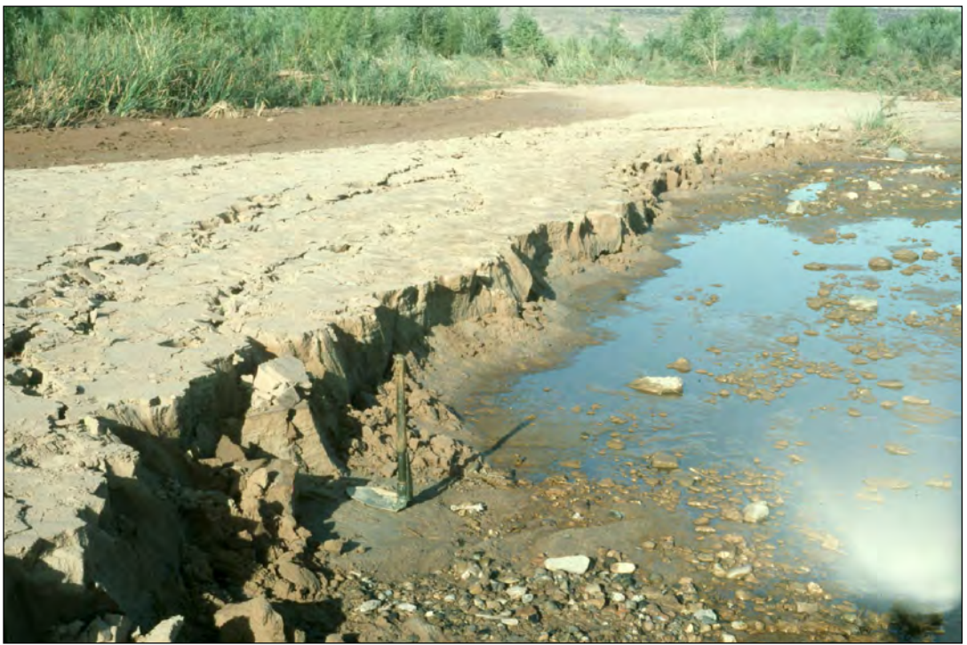
Figure 2. Lateral spread cracking from liquefaction along the Virgin River resulting from the September 2, 1992, M 5.8 St. George earthquake. Folding shovel for scale (photo credit W.E. Mulvey).
