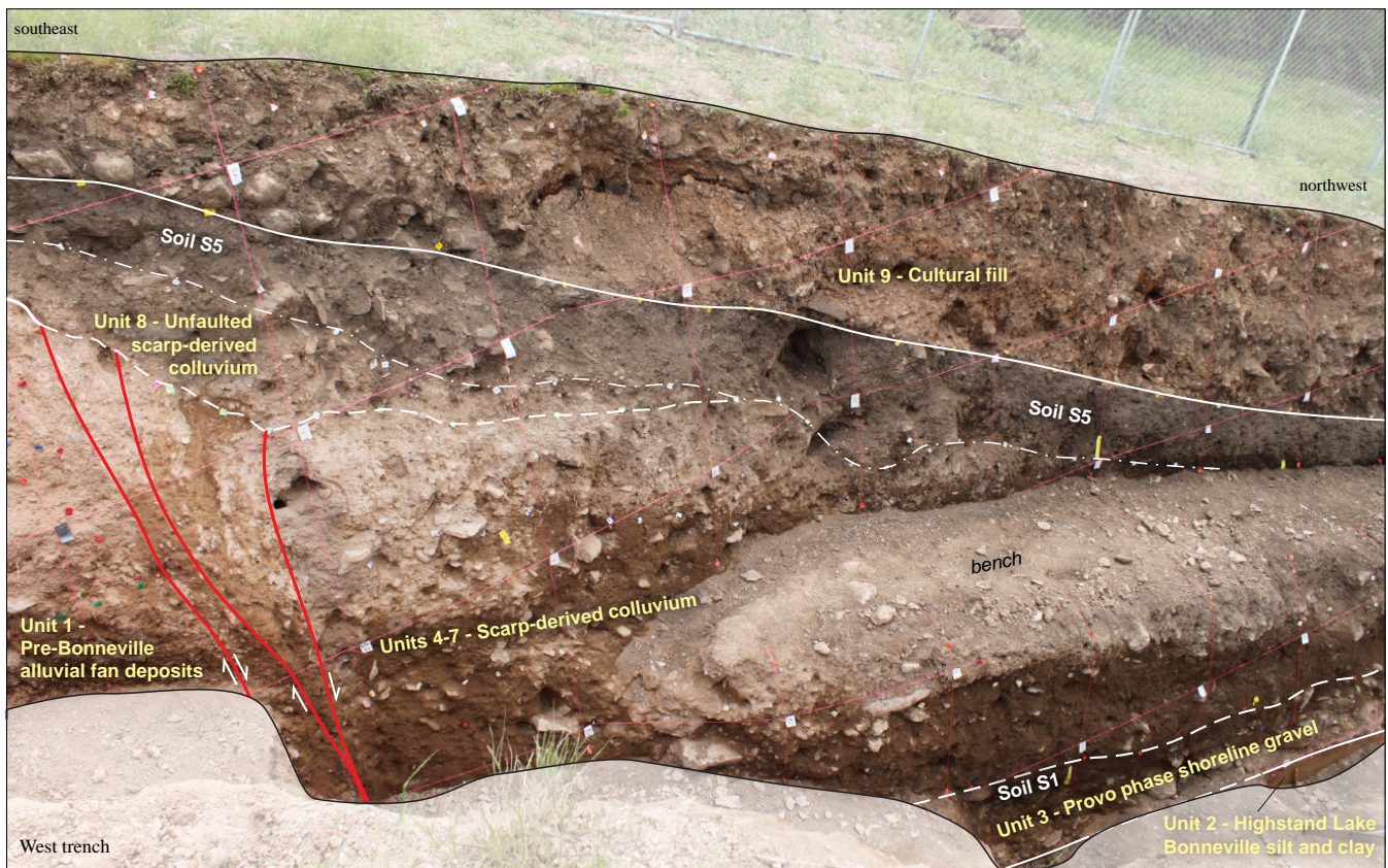
Figure 9. East Bench fault of the Wasatch fault zone (red lines) and scarp-derived colluvium (units 4–8) exposed in the northeast-facing wall of the west trench at the Penrose Drive site. S1 and S5 (buried by cultural fill) indicate prominent soil A horizons formed in Provo-phase boulder gravel and scarp-derived colluvium, respectively. See plate 1 for additional stratigraphic contacts and soils mapped in the west trench. Pink level lines form 1-m squares.
