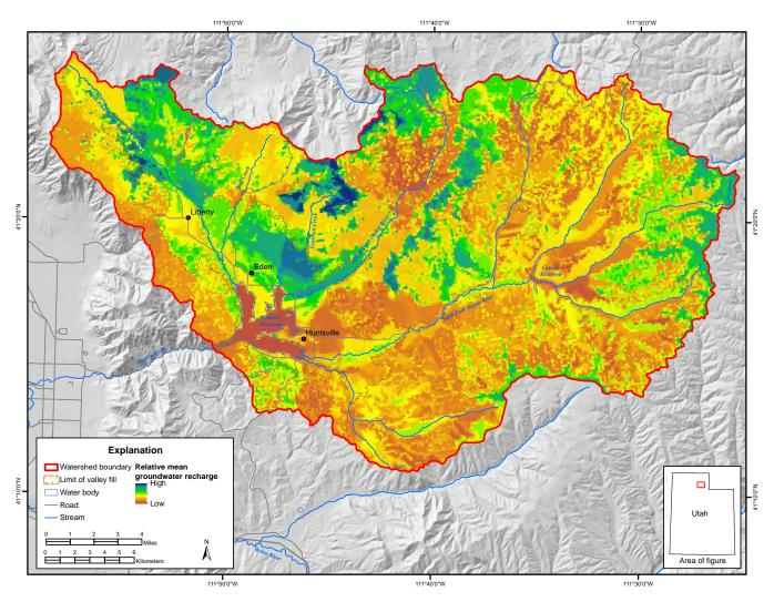
Figure 65. Relative distribution of recharge generated by the SWAT model for the Ogden Valley watershed.
