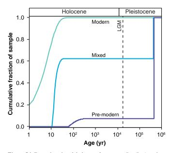
Figure 54. Examples of modeled groundwater age distributions from TracerLPM (Jurgens and others, 2012).
