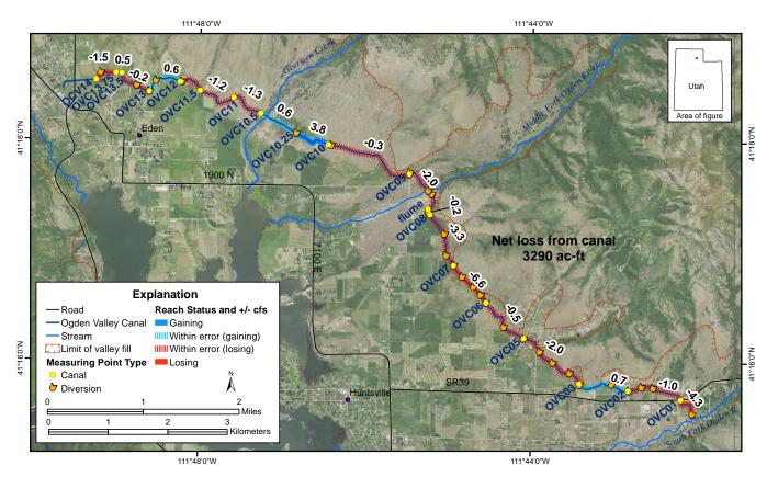
Figure 33. Gaining and losing reaches of Ogden Valley Canal, July 19, 2016.
