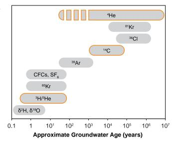
Figure 38. Approximate groundwater ages determined from different environmental tracers; age tracers used in this study are outlined.
