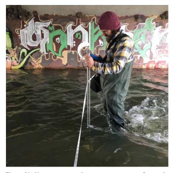
*Figure 30.* Using a current velocity meter to measure flow in the North Branch of the South Fork Ogden River.
