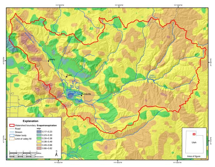
Figure 64. Distribution of relative evapotranspiration (ET) from averaged MODIS data.
