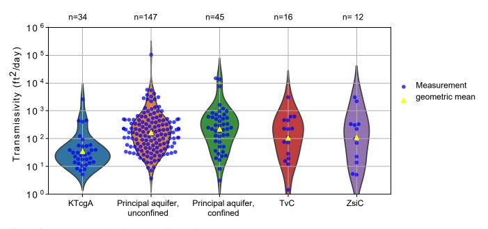
Figure 18. Transmissivity values for Ogden Valley aquifers.
