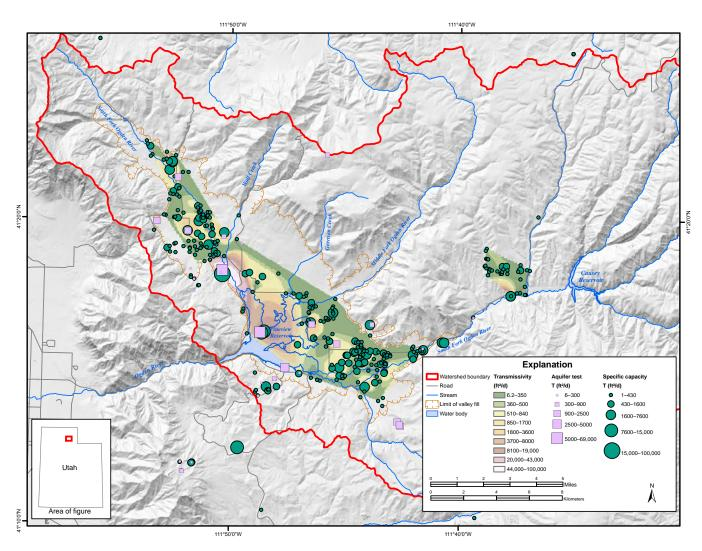
Figure 19. Distribution of transmissivity in Ogden Valley aquifers.
