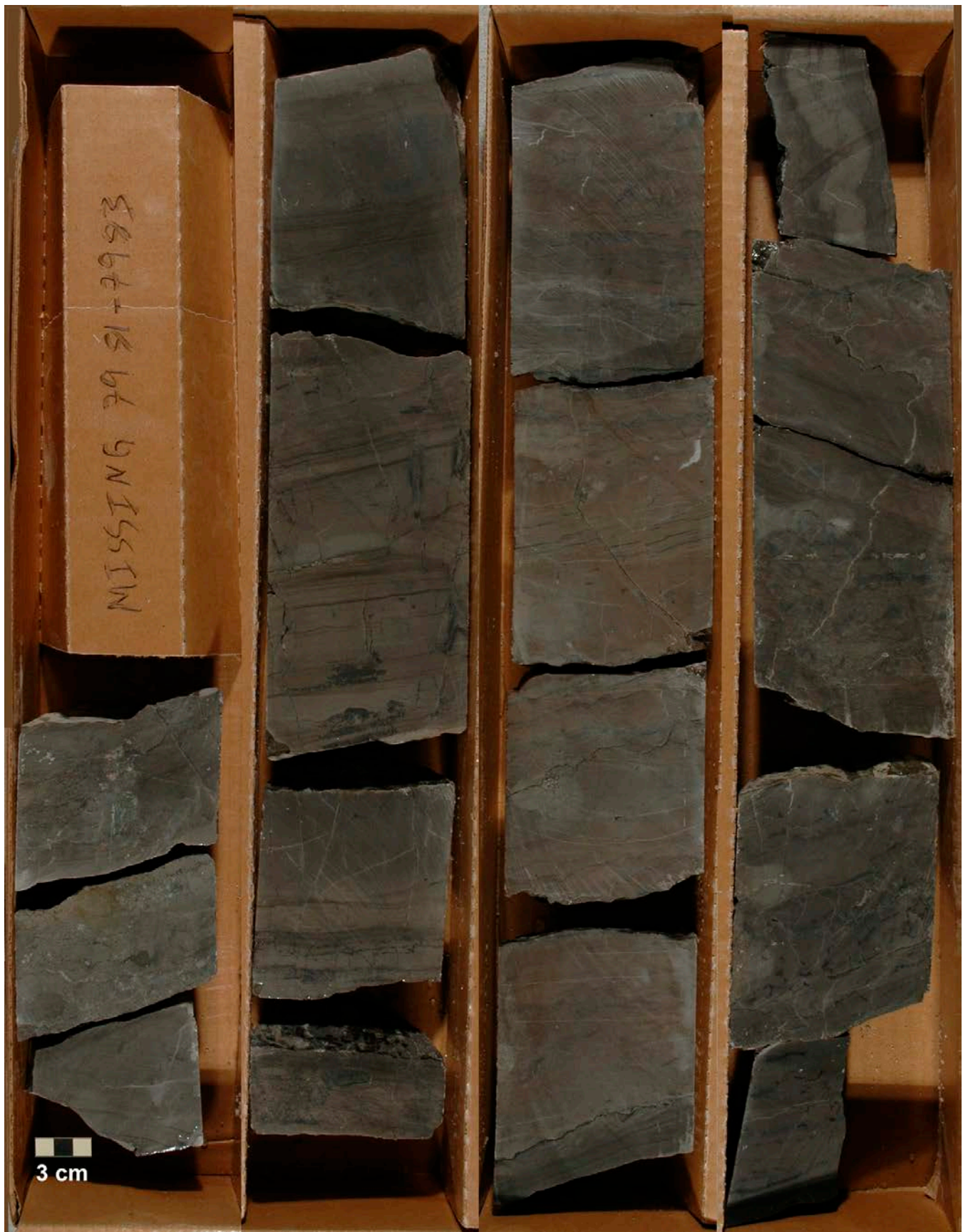
Figure 96. Stromatolitic laminations bound by lime mud. Note desiccation features and microfractures. Black bitumen lines open pores and fractures. Lisbon No. B-610 core (figure 93), 2433 to 2435 meters (7983–7990 ft).
