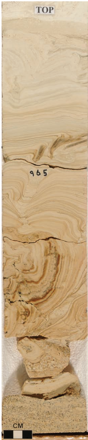
Figure 9. Stromatolites in the subsurface of the Green River Formation, Uinta Basin. (A) Large stromatolite domal head; Skyline 16 research core, eastern Uinta Basin; 294.0 to 294.4 meters (964.5–966.0 ft). (B) Close-up photomicrograph of well-laminated, dense microbial (stromatolitic) head; Federal No. 15-24B core West Willow Creek field, 1455.2 meters (4774.5 ft) (plane light).
