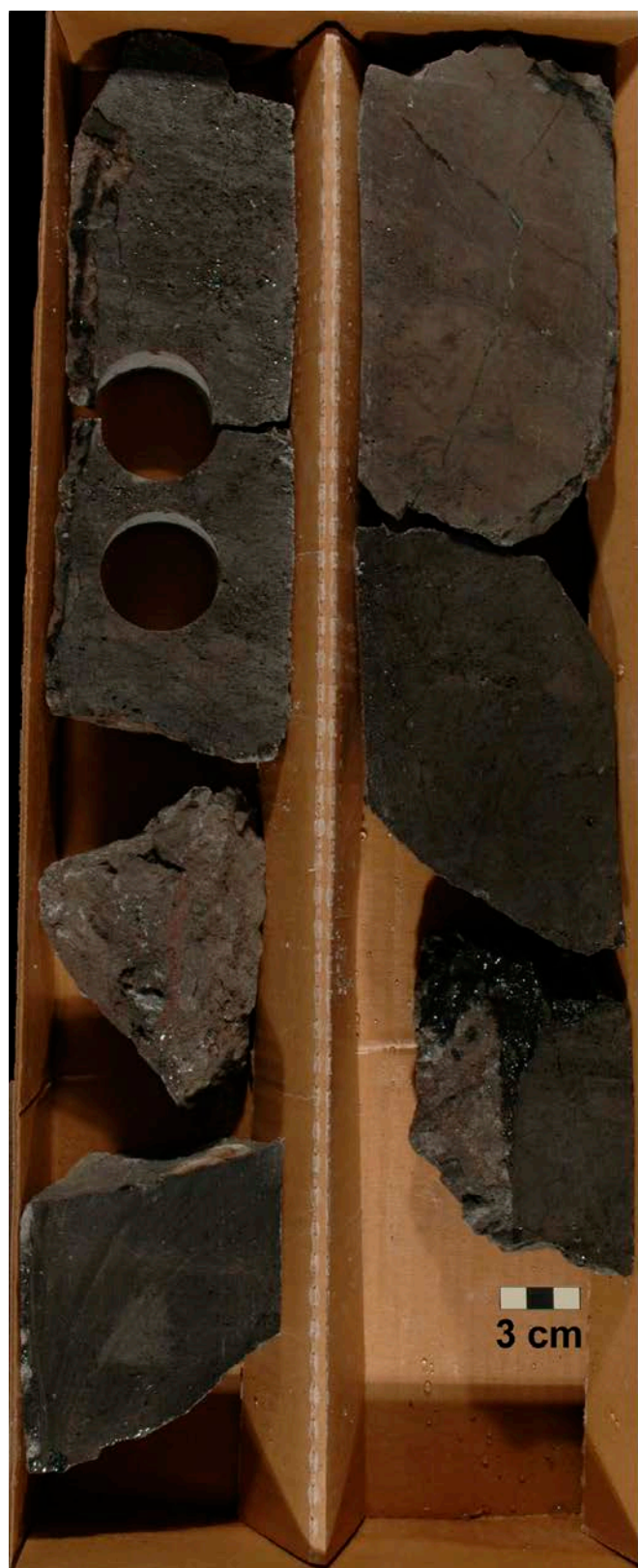
Figure 95. Stromatolitic boundstone/bindstone dominated by muddy fabrics. Note laminated rip-up clasts; the black areas are bitumen-lined pores. Lisbon No. B-610 core (figure 93), 2395 to 2396 meters (7858–7862 ft).
