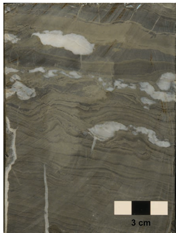
Figure 63. Microbial mudstone displaying laminated stromatolite structures, Rich Member, UPRR No. 3-3 core, 2741.2 meters (8993.6 ft); core plug analysis: porosity = 2.7%, permeability = 0.22 mD. Note the displacive and replacive white anhydrite nodules as well as vertical fractures healed with anhydrite.
