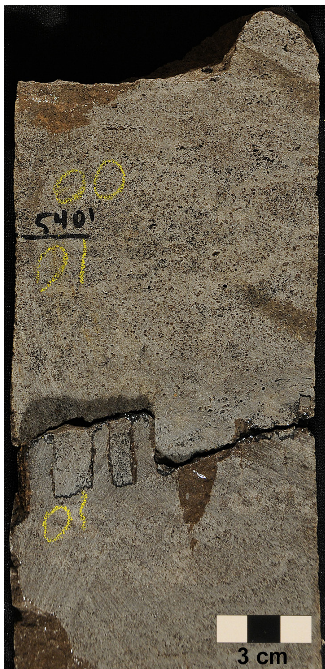
Figure 88. Porous thrombotic grainstone. Note black bitumen lining pores. Aneth Unit No. H-117 core (figure 86), 1646.2 to 1646.4 meters (5400.8–5401.4 ft).
