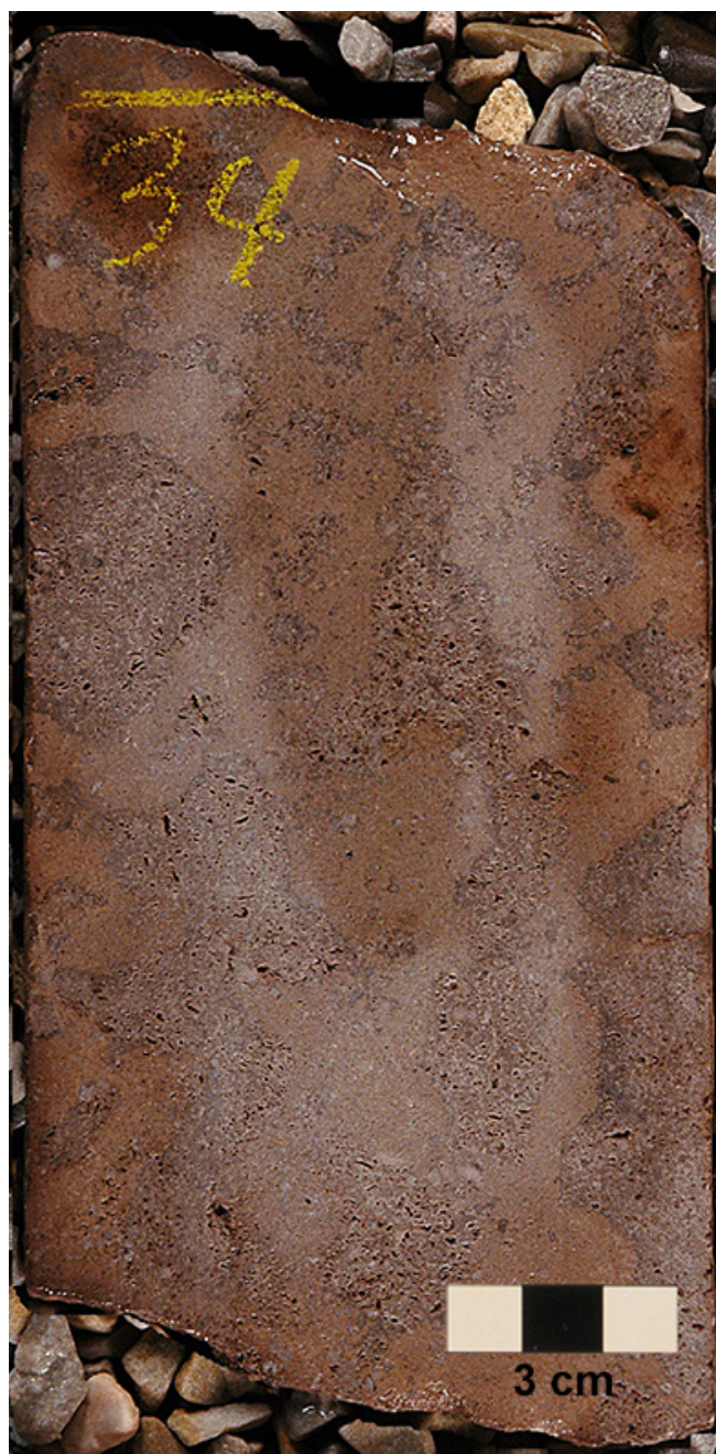
Figure 89. Oil-saturated thrombotic/stromatolitic boundstone with skeletal grainstone lenses containing fair to good reservoir quality. Aneth Unit No. 27-C-3 core (figure 86), 1747.7 to 1747.9 meters (5734.0–5734.5 ft).
