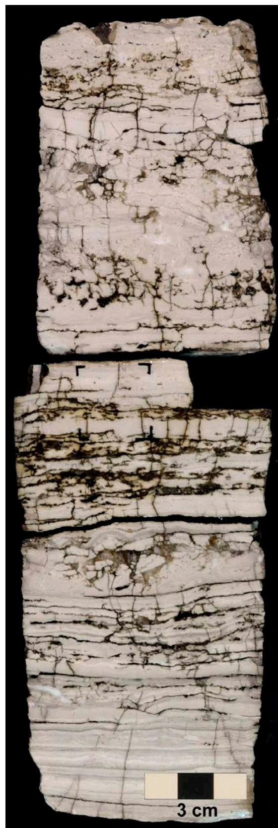
Figure 79. Thrombolites and cryptalgal laminites in the K-2 zone of the Timpoweap Member from the Upper Valley Unit No. 4 core. (A) Small thrombolite with oil staining; 1943.9 meters (6377.5 ft). (B) Flat cryptalgal (microbial) laminites with desiccation features, vertical fractures, and some minor anhydrite; 1953.6 meters (6409.5 ft).
