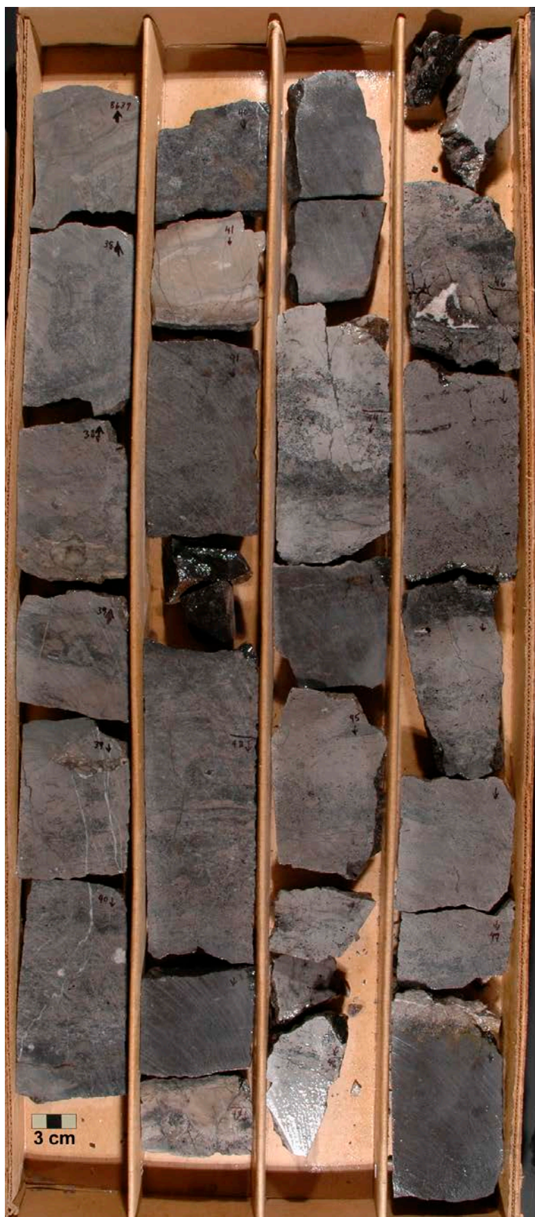
Figure 97. Stromatolitic packages alternating with rip-up clasts and eroded heads. Silicification of thin intervals can be seen in lighter rocks; bitumen lines some of the open pores and fractures. Lisbon No. B-816 core (figure 93), 2633 to 2636 meters (8637–8648 ft).
