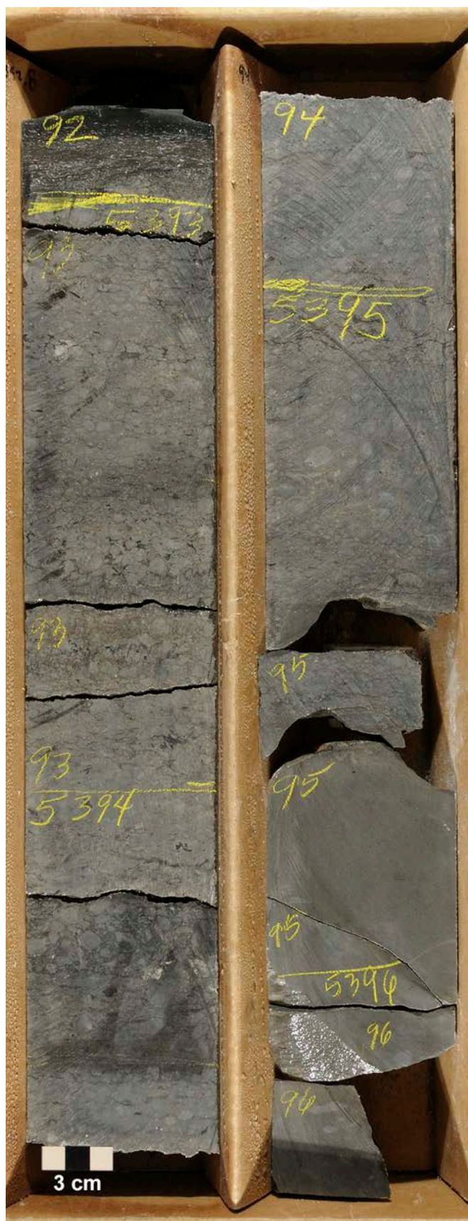
Figure 90. Oncolitic rudstone/floatstone with very poor reservoir quality. Aneth Unit No. H-117 core (figure 86), 1643.7 to 1644.6 meters (5392.8–5395.7 ft).
