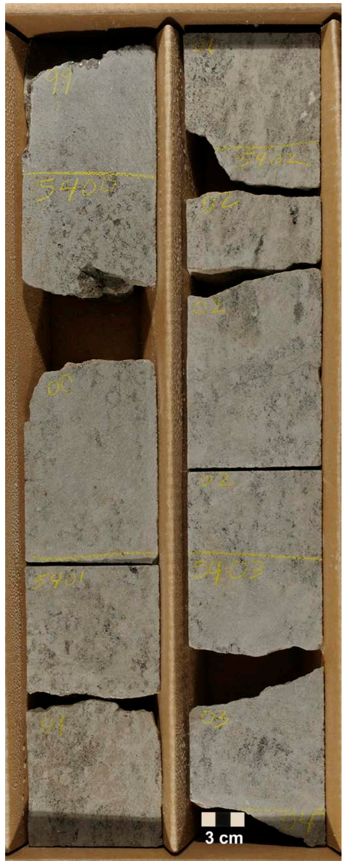
Figure 87. Small digitate stromatolites encased in skeletal/oolitic grainstone with good reservoir quality. Aneth Unit No. F-317 core (figure 86), 1645.8 to 1646.6 meters (5401.5–5402.1 ft).
