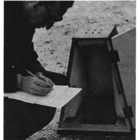
Bruce Kaliser records reading on strain gauge. Instrument spans old but reactivated landslide scarp; was operative March through August of this year. Photo courtesy of Henry L. Dequasie.
