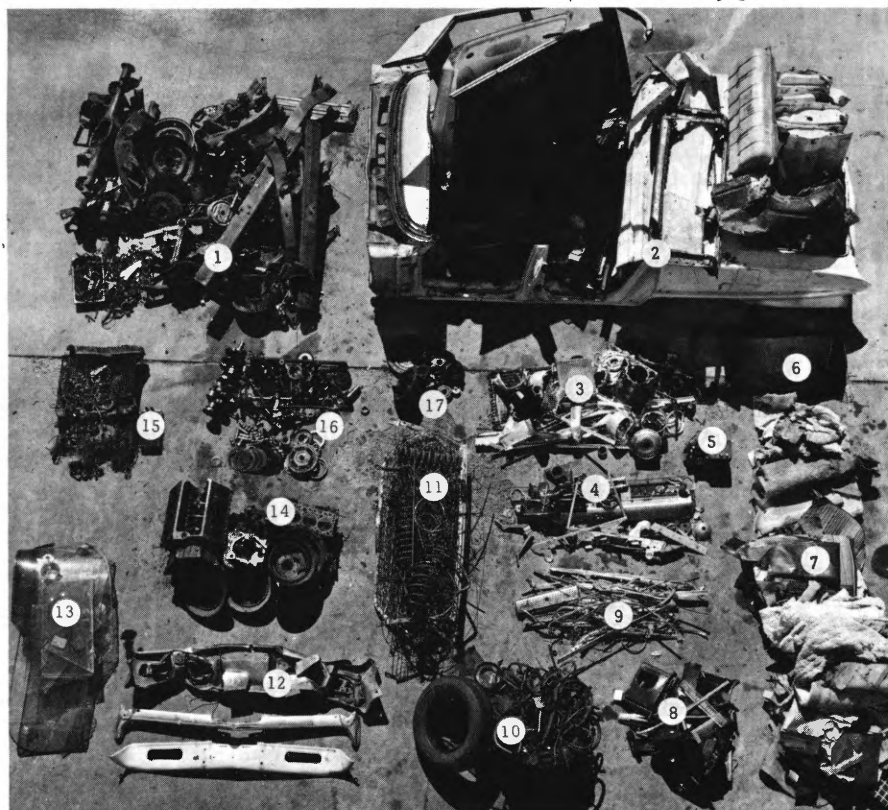
Disassembled parts from a 1961 Oldsmobile. (1) heavy steel, plus 1/8-inch thickness; (2) light steel, minus 1/8-inch thickness; (3) aluminum; (4) zinc (die cast); (5) lead (battery); fiberglass, noncombustible; (7) textiles and plastics, combustible; (8) molded paper and fiberboard, combustible; (9) light steel, minus 1/8-inch thickness, nickel-chromium-plated; (10) rubber, combustible; (11) spring steel; (12) heavy steel, plus 1/8-inch thickness, nickel-chromium-plated; (13) glass; (14) cast iron; (15) copper and brass; (16) hardened iron, and (17) cast steel. Photo courtesy U. S. Bureau of Mines.
