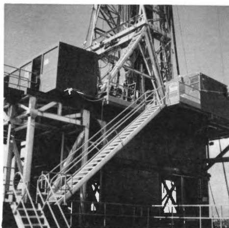
New, modern and well equipped electric drilling rig. The rig has a 26-foot substructure (left), and measures roughly 142 feet from floor to crown (right).
