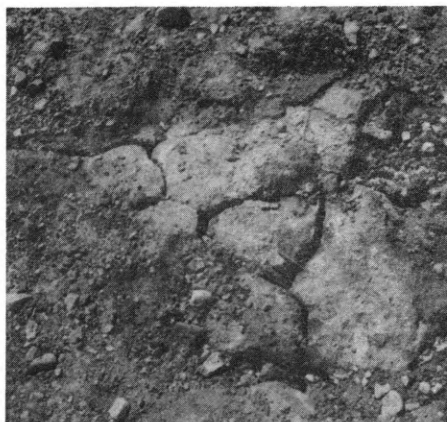
Site exploration for a city sewage lagoon uncovered jointed volcanic rock beneath an irregular veneer of fanglomerate material. A water injection test into the volcanic horizon was readily accepted. This indicated the terrain was unsuitable for its intended use. This is an example of a problem which can arise if the geologic setting is ignored.
