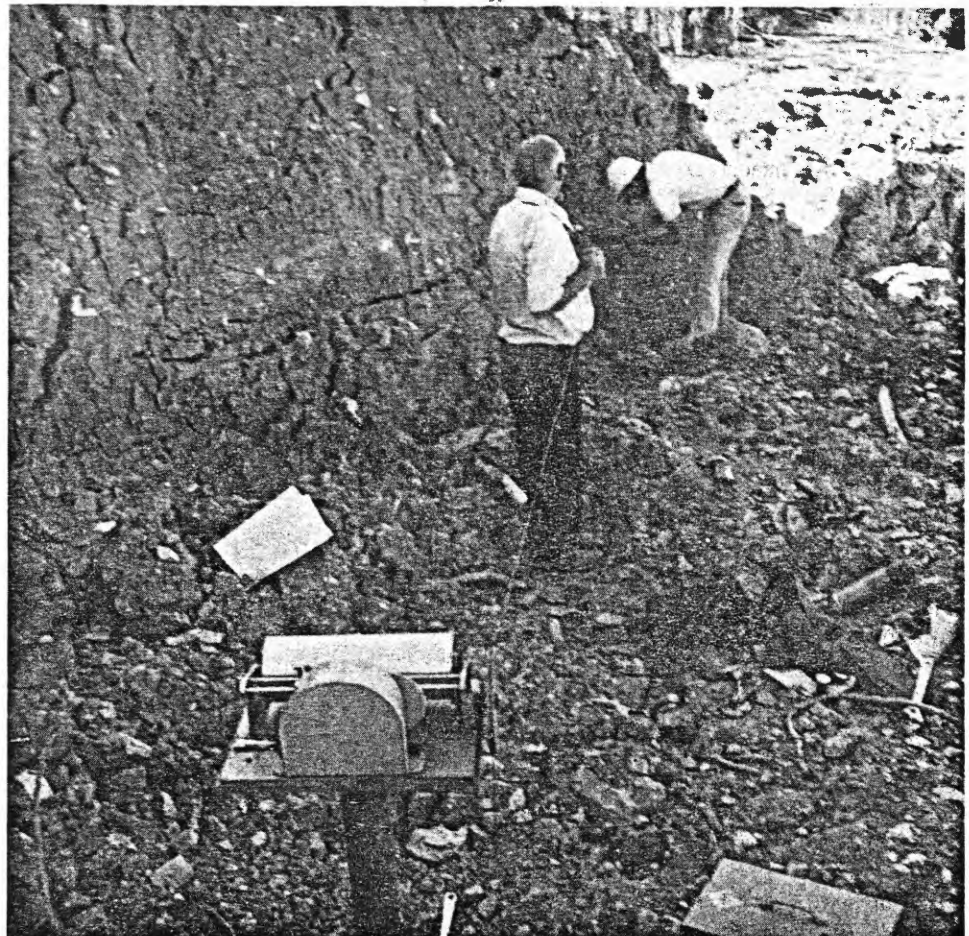
Top: En echelon fracturing of earth embankment of Cottonwood Dam affected by sliding (August 1975). Bottom: Installation of continuous recording extensometer across eastern boundary fracture near point where Manti aqueduct was severed in 1974. End of wire is attached to a pole driven into uplifted pressure ridge (August 1975). (UGMS photos) (continued on page 6)
