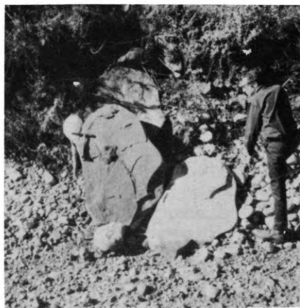
Large gray slab of sandstone (left of center) slumped about 10 feet into dry bed of Farnsworth Canal 3 miles south-southeast of Moon Lake after earthquake. White stain (below level of pick on slab) marks high water level of canal. Slab is not stained in contrast to slab at right and cobbles and boulders right and left. White object to left of pick is hard hat.
