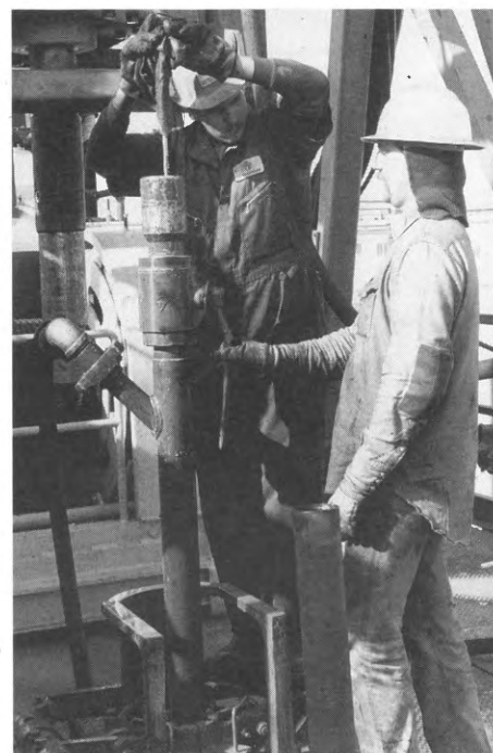
The drilling crew retrieves the inner barrel after a 20-foot (6 m) coring run.
