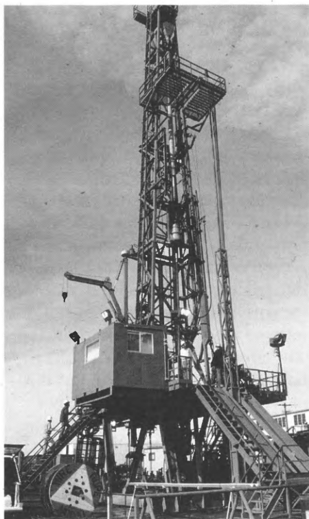
The rig, fabricated by Kremco of northern Utah, can drill or core to 14,000 feet (4,300 m). The rig floor is 25 feet (5 m) above the ground and the stand of drill pipe in the monkey boards is approximately 60 feet (18 m).
