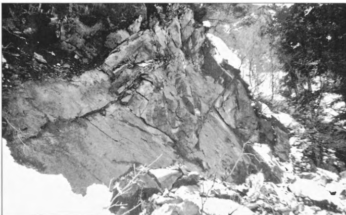
Source outcrop of rock fall showing intersecting fractures. Rock-fall material detached from dark area at upper left corner of outcrop. Outcrop is approximately 15 feet high.
