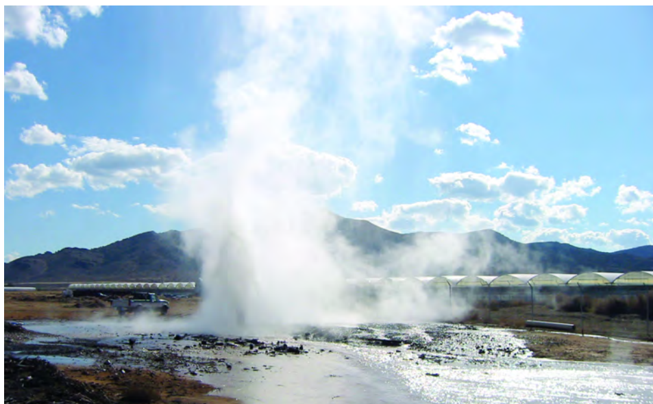
Geothermal well testing at Milgro Nurseries commercial greenhouse facility at the Newcastle geothermal area, Iron County, Utah. Since 1992, Milgro's operation has grown to include nearly 1.1 million square feet of greenhouses, heated directly from a geothermal reservoir, that produce 13 million potted plants and cut flowers annually.
