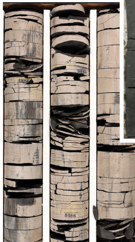
Well core of typical Gothic shale (Paradox Formation). Slabbed core (inset) shows vertical fractures. Effective gas production depends on interconnected fracture networks.
