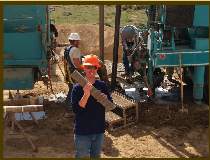
UGS geologist Andrew Rupke "catching" core as it is brought to the surface.
