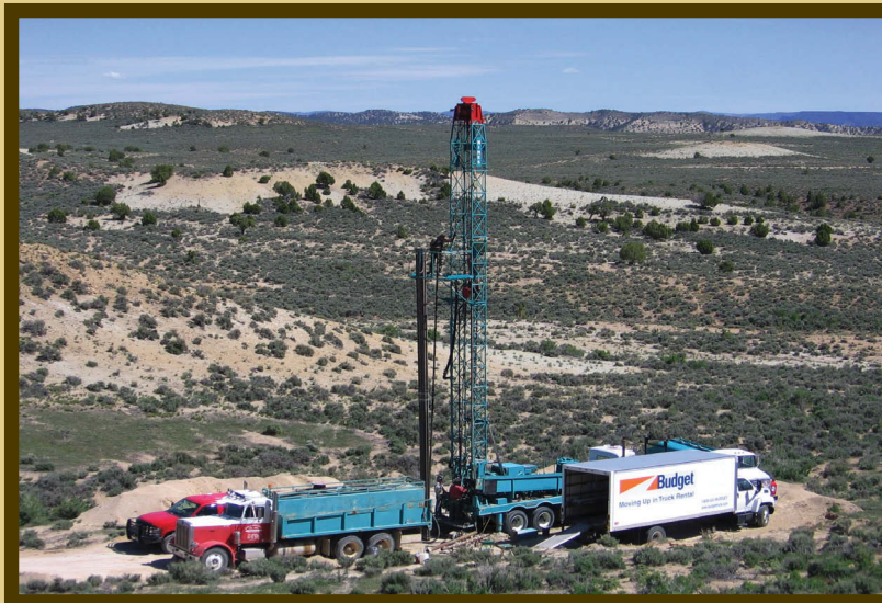
Drill rig used to recover the Skyline 16 core in the eastern Uinta Basin.
