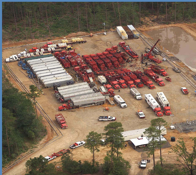
Aerial view of typical frack equipment operating in the southern U.S. Photo courtesy of Halliburton.
