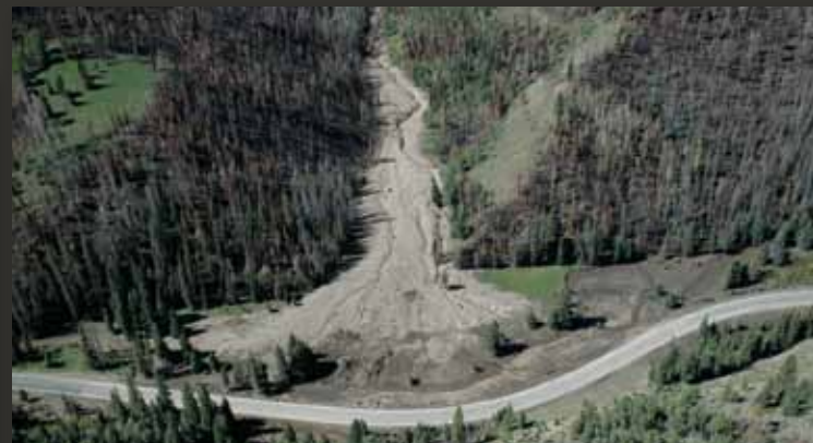
A September 1, 2012, fire-related debris flow covered most of the Mill Canyon alluvial fan and deposited sediment into Huntington Creek. State Route 31 is at the bottom of the photograph (photo courtesy of Emery County Sheriff's Department).
