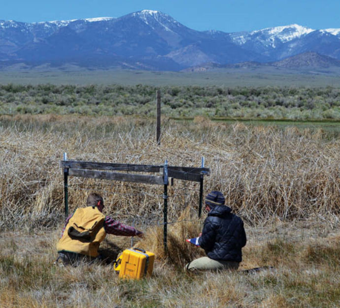
Utah Geological Survey researchers Rich Emerson and Diane Menuz download data from an automatic recording probe in a shallow wetland well on the edge of Pruess Lake in southern Snake Valley. Water level data are recorded every hour year-round and can be used to determine natural seasonal and annual fluctuations and responsiveness to groundwater manipulations.
