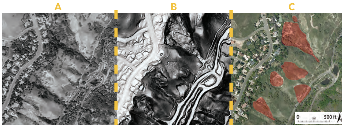
Three views of the historically active City Creek landslides that lie between Capitol Boulevard and the City Creek Canyon floor. (A) In the 1990s aerial photograph, the landslides are obscured by brush on the canyon wall, whereas in the new (B) 0.5-meter 2013–14 LiDAR slopeshade map the landslides and their geomorphology are clearly visible. (C) The newly remapped landslides are shown in red on the 2009 aerial photograph.
