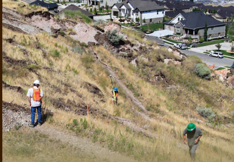
UGS engineering geologists inspecting landslide features and monitoring landslide movement with GPS equipment at the Parkway Drive landslide, North Salt Lake (photo courtesy of Adam Hiscock).
