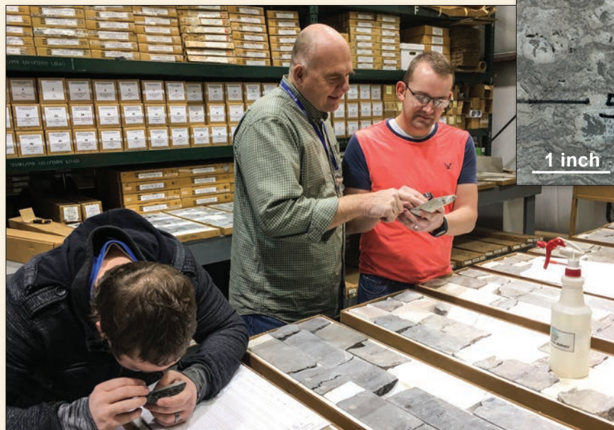
Graduate students and their professor from Brigham Young University examining newly donated Greater Aneth cores as part of their thesis research. Inset is an example of Paradox Formation core from Greater Aneth field well, McElmo Creek No. J-15, showing the lower producing reservoir. The environment of deposition of this sample was a reef-like buildup of algae in a shallow, warm sea.
