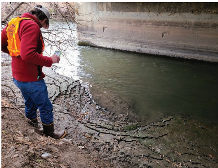
Minor ground shaking-related lateral spreading observed along the Jordan River.
