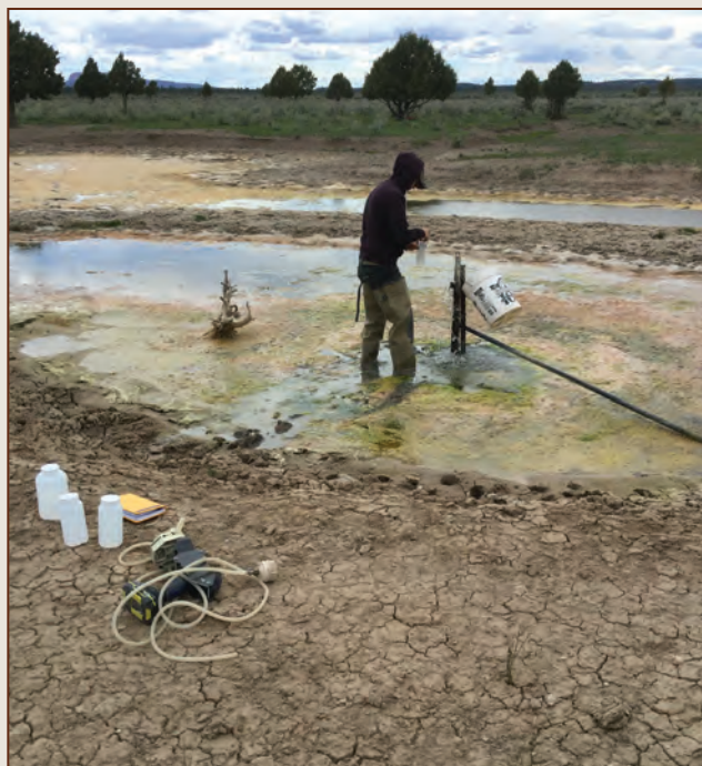
UGS employee sampling a well for solute chemistry, nitrate, and radiogenic isotopes.
