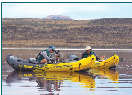
Elliot Jagniecki and Andrew Rupke investigate the halite saturation state of the north arm of Great Salt Lake by sampling and testing the lake brine in 2021.
