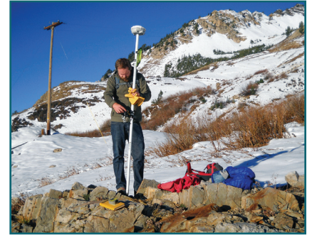
Greg McDonald performs a GPS survey to map debris flow deposits in Little Cottonwood Canyon, November 2010.
