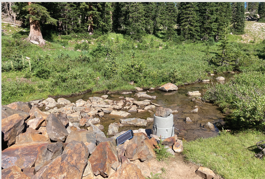
Example of an automated water sampler deployed below a rock glacier in Little Cottonwood Canyon. These programmable devices collect water samples at set intervals to monitor the chemical changes between snowmelt-dominated runoff and ice-melt-dominated runoff.
