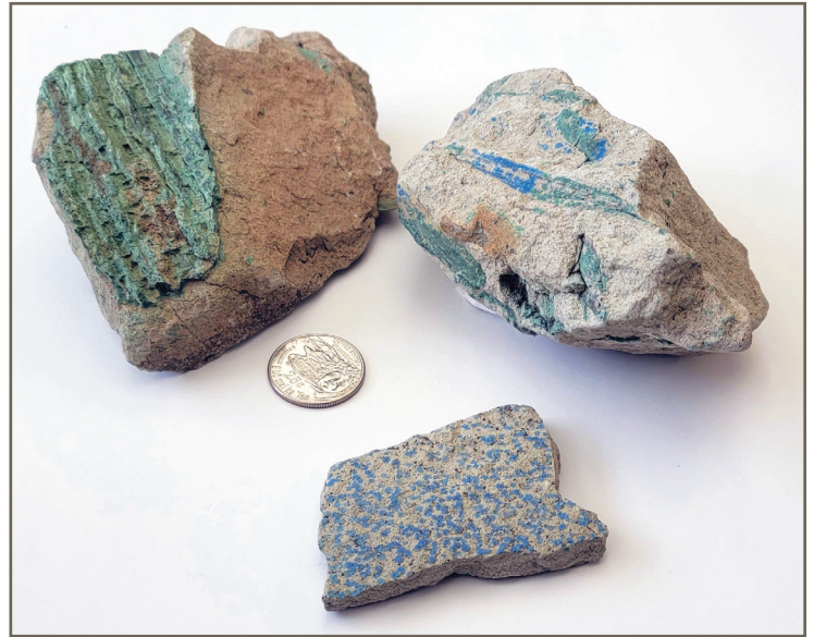
The silver minerals at Silver Reef are nearly invisible but they can occur with colorful copper and uranium minerals. Top samples—blue azurite and green malachite replacing plant fragments. Bottom sample—blue azurite “dots” on sandstone. U.S. quarter for scale.
