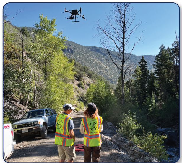
Ben Erickson and Torri Duncan launch a UGS UAV to collect digital elevation data after the 2024 Silver King Fire to support the emergency response for the town of Marysville. Photo courtesy of William Davis, Mayor of Marysville.
