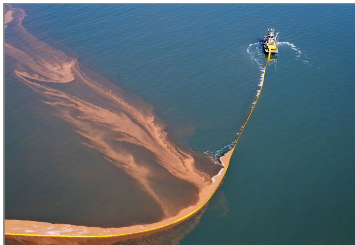
A brine shrimp cyst "slick" on open water in Great Salt Lake's south arm, measuring hundreds of feet across. Eggs concentrated from winds and currents are located by brine shrimpers, then boats corral the eggs by deploying spill containment booms and then pump them into drainable mesh sacks. The eggs are dried, processed, and packaged for distribution across the globe. Bottom photo courtesy of Utah Division of Wildlife Resources.
