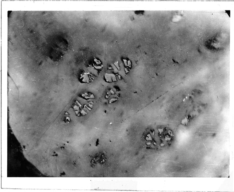
FIGURE 19. Corroded uraninite nodules in asphaltite. Light areas consist of high concentrations of submicroscopic granules of uraninite \times 1500 . (after Hausen, 1957)
