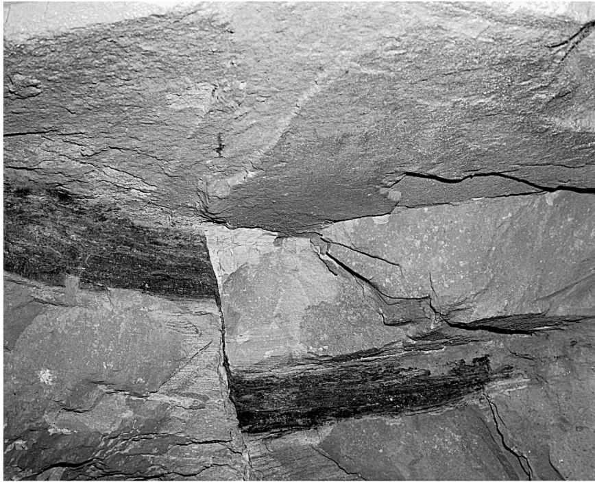
22 FIGURE 14 Post-Ore Fault in Lopez Incline Mine. Dark bands are uranium ore.
