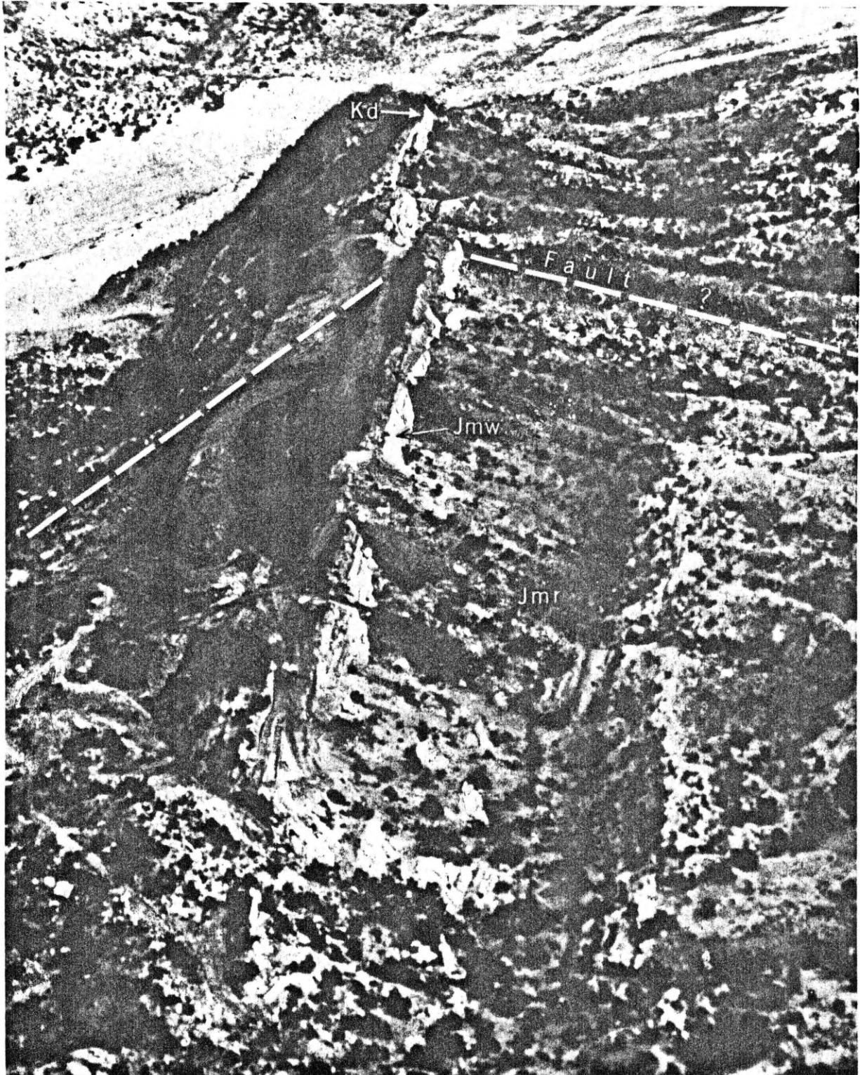
AERIAL VIEW, LOOKING NORTH, OF HOGBACK NO. 4 MINE, MCKINLEY COUNTY, N. MEX. Dakota sandstone (Kd) and Westwater Canyon (Jmw) and Recapture members (Jmr) of the Morrison formation.
